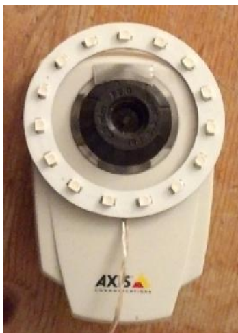
FIGURE 7.6 An “angel eye” ring light mounted on a camera. Note the piece of duct tape used to keep the adjustable focus from being accidentally adjusted.
