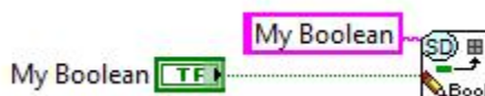
FIGURE 8.2 Putting a Boolean value into the network table. Note the pencil to indicate that we are writing data.
