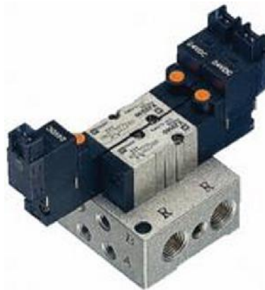
FIGURE 5.17 A Single solenoid valve (one orange dot) and a Double (2 dots). These valves are from SMC. They don't look exactly like what you are likely to find in your team's box of random pneumatic stuff, but are close enough. If you press on the dot, the valve will act as if a voltage has been applied to that coil.
