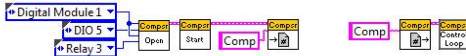
FIGURE 5.16 Left: code to set up the compressor. In this example, the DIO channel for the pressure switch and the relay channel for the Spike relay are both connected to the same Digital Sidecar, but they could be on separate ones. Right: code to run the compressor, which goes in Periodic Tasks. Note that the Control Loop is already a loop, and should not go inside a While Loop.
